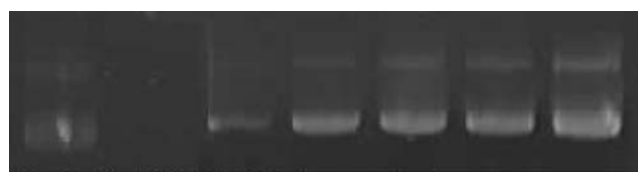
Fig. 4. Agarose gel (1%) assay of fluorescent EthBr intercalated in pEGFP, lipoplex formation with N 1 ,N 12 -dimyristoyl spermine 6 at N/P ratios 2–12 progressively retards gel permeation.
